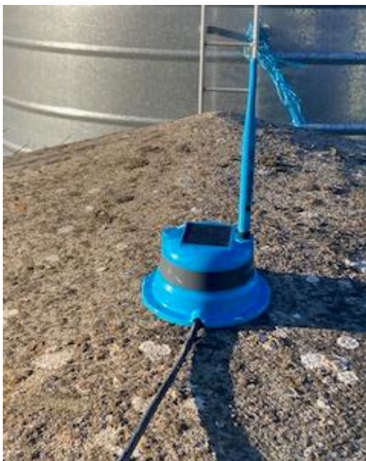
Figure 1: Tanks 360 Tank Level monitor
