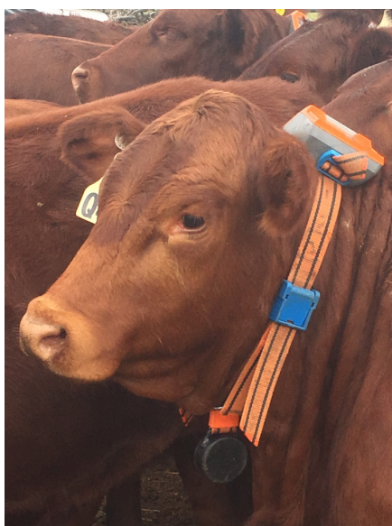
The eShepherd® pre-commercial neckband prototype fitted to cattle in the Eden Valley trial.
