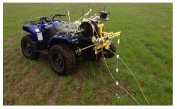
A two line temporary electric fence being erected using Rappa Supporting Partners:
