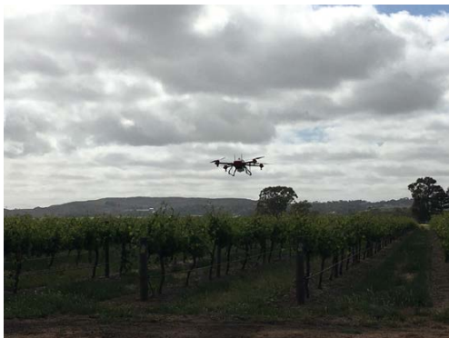
P20 2017 Crop Protection UAV tracking, spraying and approaching the end of a vineyard row.
