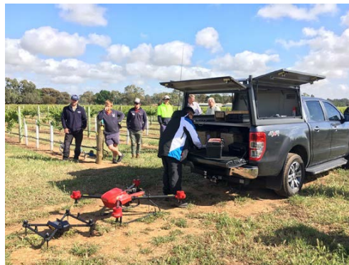
Revolution AG's "techy" Alex unloading both the C2000 Surveying drone and the P20 2017 Crop Protection drone with all associated GNSS RTK Positional guidance equipment.
