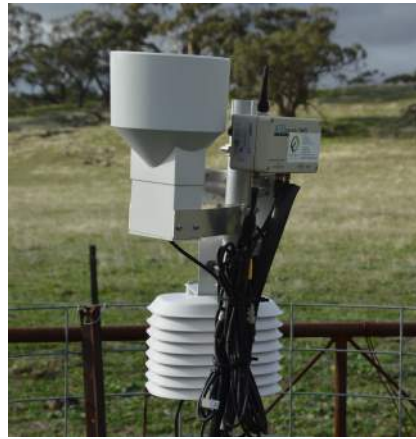
The technology used to collect soil moisture, rainfall, temperature and humidity data for BIGG's Soil Moisture Monitoring Project
