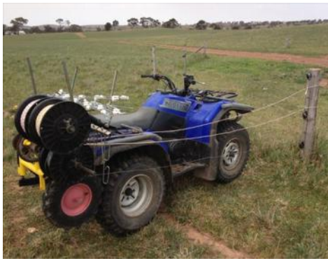
The Rappa system in action rolling up the temporary electric wires. The system is now ready to be used around the district!
