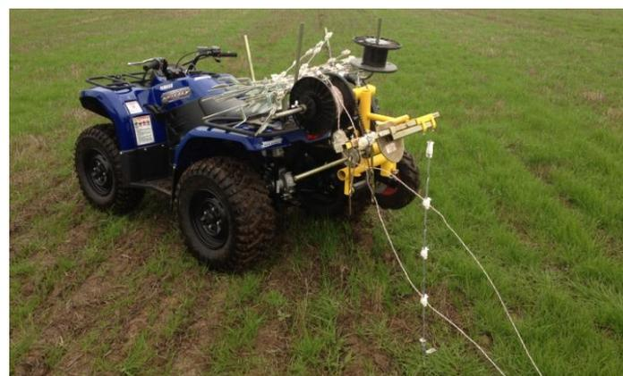
*A two line temporary electric fence being erected using Rappa*
